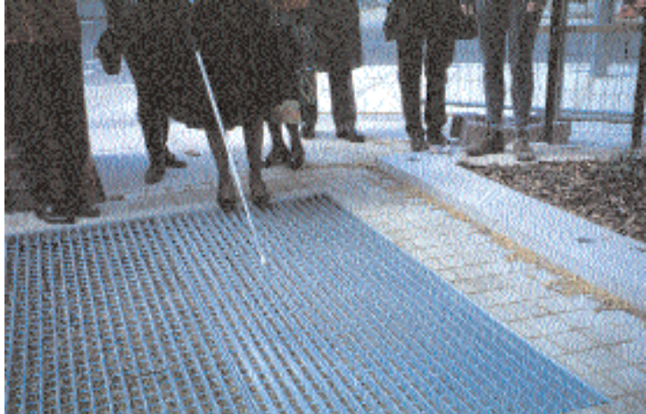
Graduate course 1996 – disabling dog grids being tested by a blind person.
