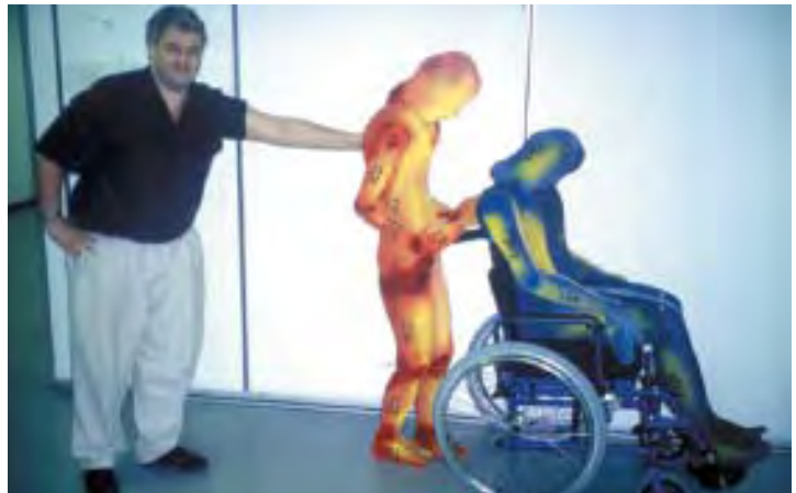
Anthropometric dummies can be constructed to aid the appreciation of a diverse range of user abilities.
